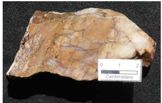
Figure 10: KRS207729: 3.11g/t Au and 0.9g/t Ag, intensely silica-illite/sericite and haematite-limonite oxidised, hydraulic vein breccia composed of basement and ghosted interlocking crystalline quartz clasts, re-healed by silica (Float)
