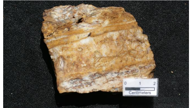
Figure 8: KRS207747: 3.23g/t Au, 1.8g/t Ag and 4040ppm As, intensely silica-illite ± pyrite altered sheared leucogranitic basement, cut by hydraulic brecciated and mesocrystalline quartz veinlets in an interlocking crystalline quartz vein matrix (Float)
