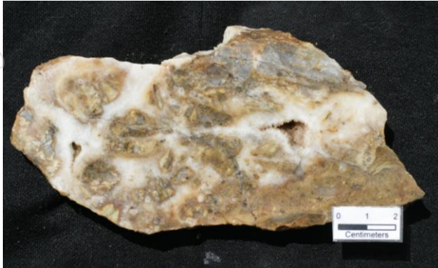
Figure 7: KRS207708: 3.56g/t Au and 0.2g/t Ag, hydraulic vein breccia, composed of milled granite fragments, set in an interlocking crystalline quartz matrix, with partially crudely cockade-comb banding (Float)
