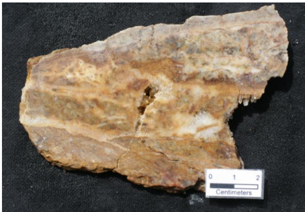
Figure 9: KRS207702: 3.17g/t Au, 0.4g/t Ag, and 1770ppm As, intensely silica-illite/sericite ± pyrite altered hydraulic breccia and crystalline to mesocrystalline quartz vein re-healed granite/gneiss (Float)
